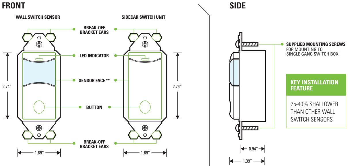
\*\* SENSOR FACE IS FIELD REMOVABLE IN ORDER TO CHANGE COLORS. CONTACT FACTORY FOR ADDITIONAL FACES
